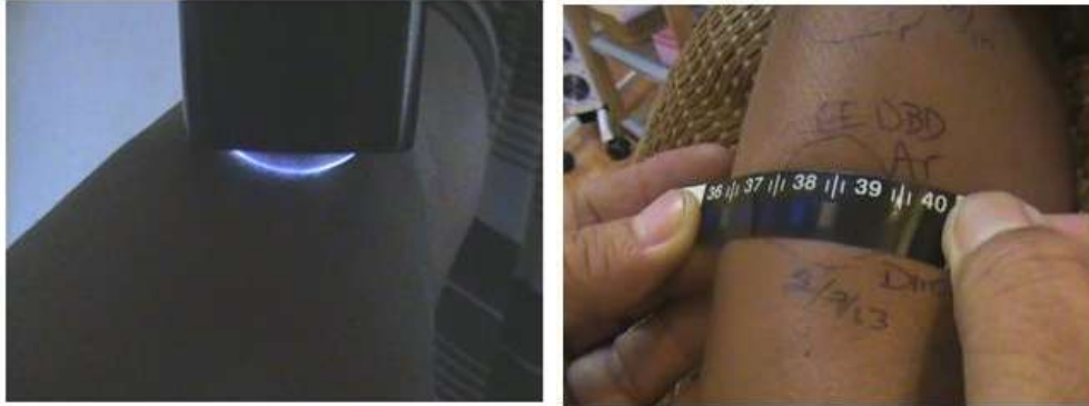
Fig. 2. CAP was applied to arm skin and temperature strip was measured afterward, from left to right. The setting was 5/50 at 24°C 50% RH [9].
