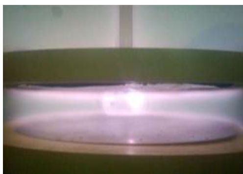
Fig. 8. RF PECVD system for a-C film synthesis on PS dishes.
