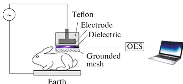
**Fig. 1.** The scheme of plasma treatment of rabbits (OES—optical emission spectroscopy).
