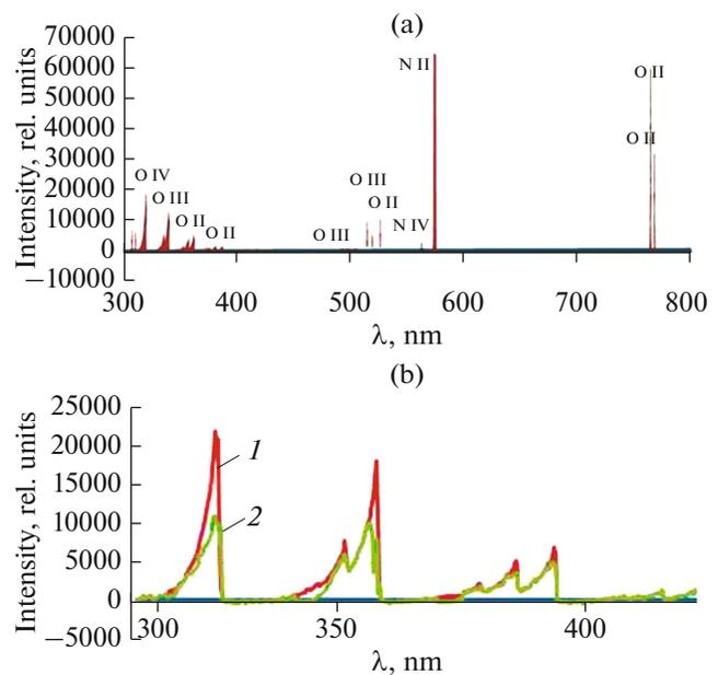
Fig. 3. The optical emission spectroscopy of the FE-DBD plasma: (a) the optical emission spectroscopy of the FE-DBD plasma without mesh; (b) OES analysis of FE-DBD plasma with mesh.
